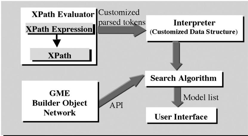
Figure 5: Architecture of the XMOS plug-in
