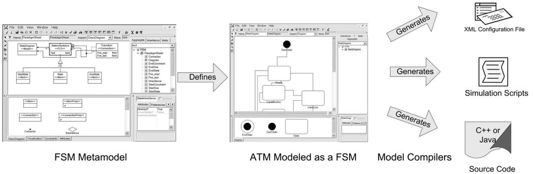
Figure 3: Metamodeling process with the GME
