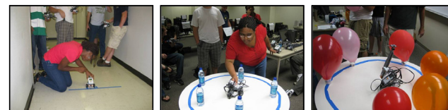
Figure 5: Students testing their programs and competing in robot challenges. Left: Homing Pigeon, robots travel out-and-back over 10 feet to their exact starting point requiring precise control of the robot. Center: Kick-The-Can challenge, robots must eliminate all the bottles in a timed event. Right: Seek-And-Pop, the robots must seek out balloons and pop them in a timed event. These events demonstrate the student's ability to solve a challenge and control their robot with a program they wrote. Competing against the other students shows the excitement of computer science and the promise of technology education and careers.
