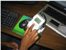
The robot is a product of LEGO. The LEGO Mindstorms NXT robot was made available to consumers in July 2006. The NXT has many unique functions and capabilities, including Bluetooth connectivity; light, reflectivity, ultrasonic distance, sound, and touch sensors; three motors; a 32-bit processor; and 256 Kbytes of Flash memory.
