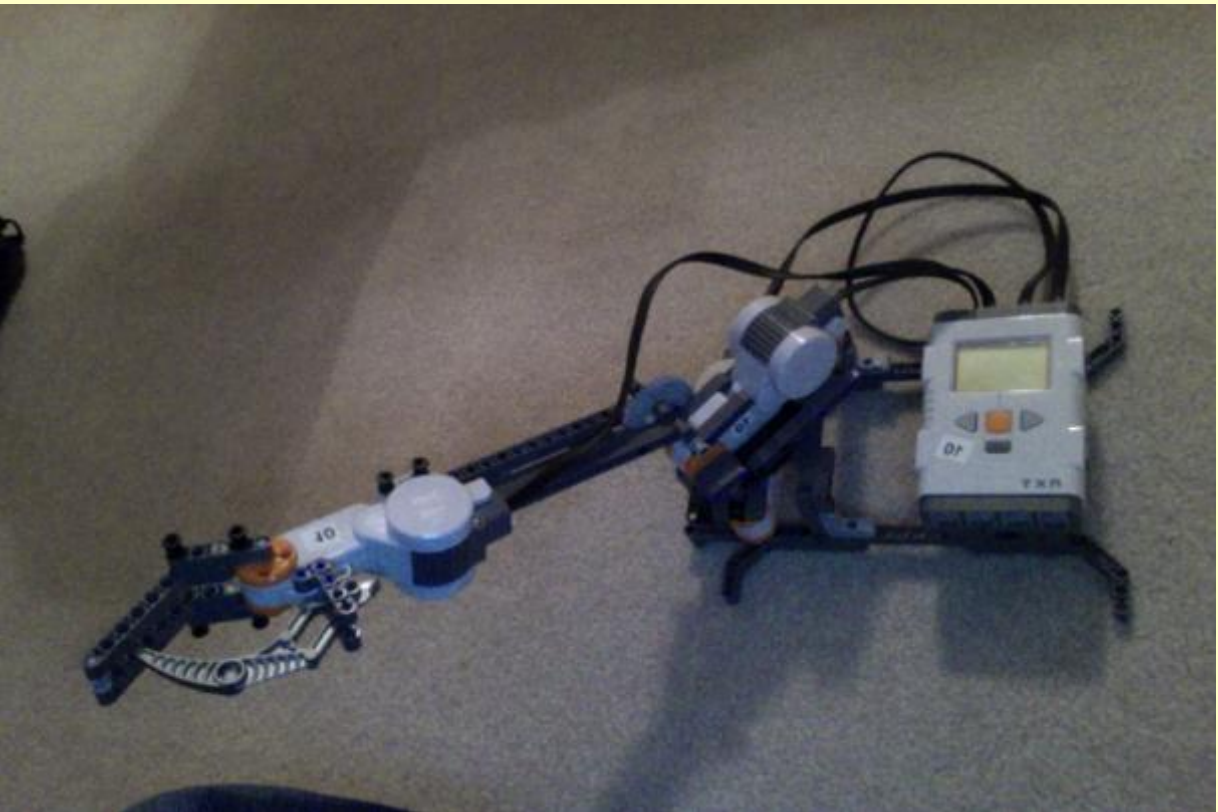
Figure 2: The robotic arm, constructed with Lego Mindstorms
