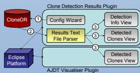
The plugin plays the role of an interface between CloneDR and the user. It performs the duties of setting up the configuration file, executing CloneDR as an external task, and displaying the clone detection results to the user.
