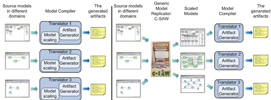
**Fig. 1.** Alternative Approaches for Scaling Models
